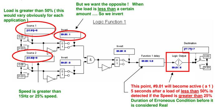
So this should do it ! Now we have an indicator bit, #9.01 that will indicate when we have a broken belt, popped chain, broken pipe or dry well etc.
