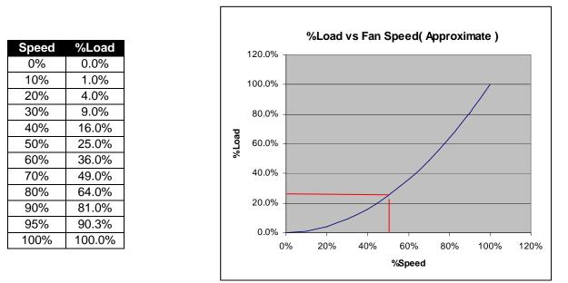
We can see that at 50% speed the load on a fan motor would be approximately 25%. If we decided that our minimum operating speed is 50% of maximum then our motor load should be at least greater than 20%- if the motor was indeed turning a fan. Otherwise we might surmise that the belt has popped off a pulley or just snapped.
